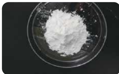
Microencapsulated Phase Change Material- no formaldehyde release, latent heat value >190J/g, from a few microns to dozens of microns in size, phase change temperature adjustable.
